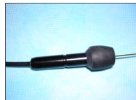
Image 6: Endoscope spring action locking mechanism
