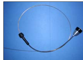
Image 4: Endoscope fiberoptic bundle
